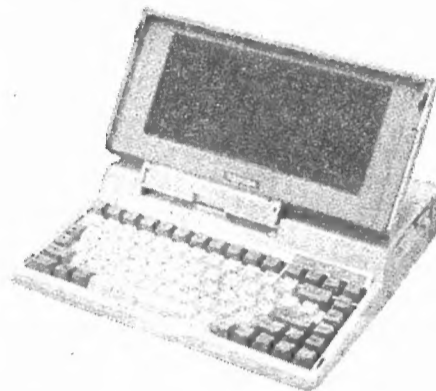
T 1200 Processador 80C86, 9.54 MHz 1Mb RAM, 1 Floppy 3,5" 720 kb, 1 Disco Fixo 20 Mb, Display LCD Supertwist, Peso 5.5 kg.
